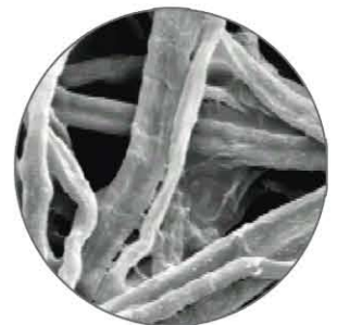
Cellulose fiber at X500 magnification
