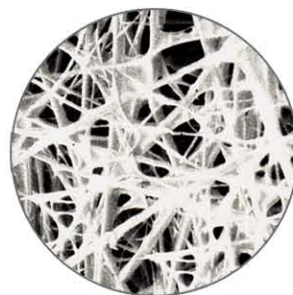
Micro-glass fiber at X500 magnification
