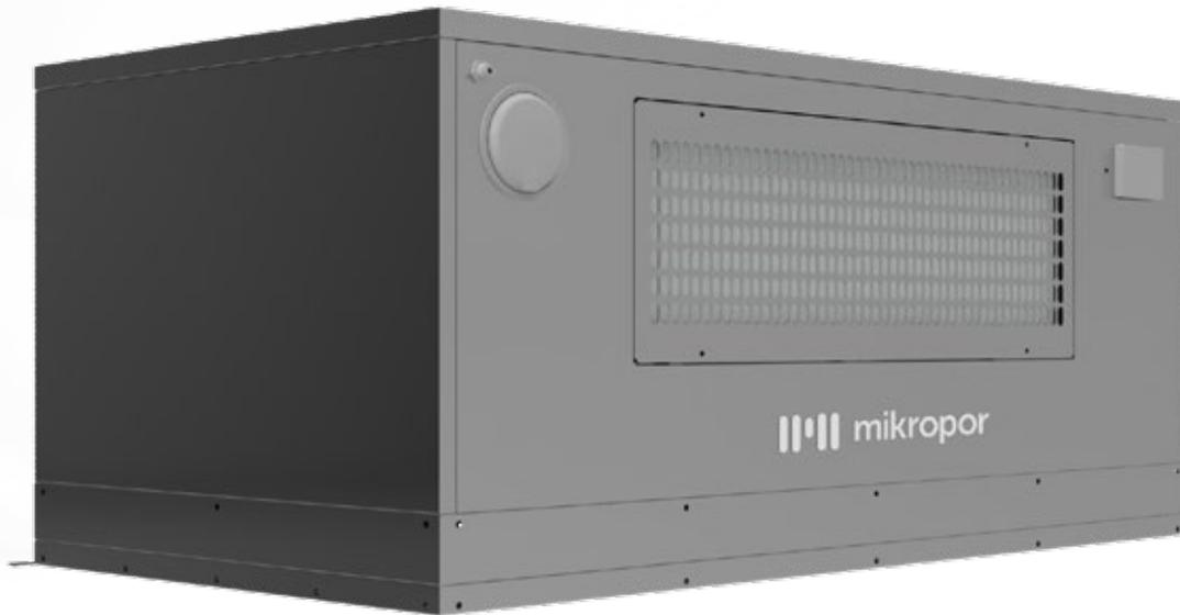
Mikropor produces Fan Filter Units with two stage filtration. Fan Filter Units ( FFU) are based on a push and pull working principle, with environmental air drawn through a G4 class coarse filter to capture relatively large particles.
