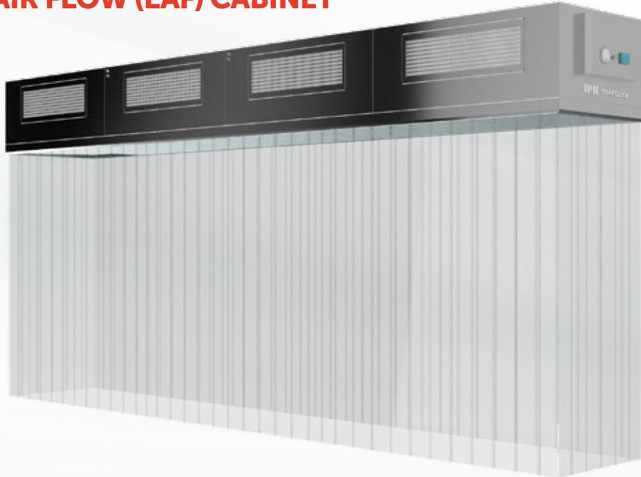
Mikropor's LAF (Laminar Air Flow) Cabinets are manufactured in accordance with ISO 14644-1. The LAF Cabinet is designed to provide a vertical air flow which is different from regular fan filter units. LAF Cabinets are isolated on the down flow area with plastic curtains. With the assistance of positive pressure inside this isolated area, any air outside this unit will not be able to get inside and cause contamination.
