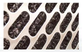
To protect the condensers all MCHILL chillers include progressive composite fiber mesh filters which can be easily removed for service and cleaning. Stainless steel frame avoids corrosion even when the filter is washed with water or other washing fluids.
