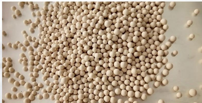
In order to achieve high purity oxygen production special zeolite granules are used. Zeolite, a microporous aluminosilicate mineral, is used as a molecular sieve and as an adsorbent of a wide variety of molecules.
